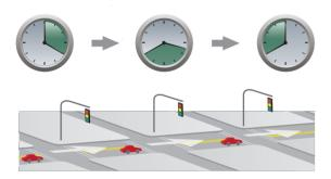
Imagine that each traffic signal has a clock with a second hand. Each signal's second hand is staggered from the others to allow travel time for each direction.
